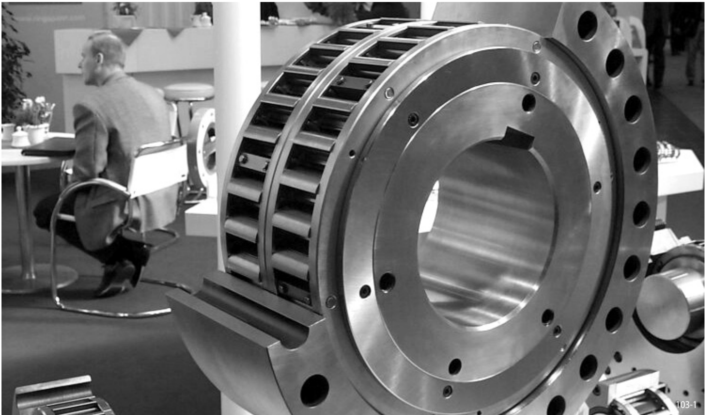
Backstop FXM 2.410 - 100 UX for the primary cooling water pump in a nuclear power station. Required torque 500 000 Nm. Speed 1 485 min -1 . In service since 1996. Manufactured and tested with extensive documentation from RINGSPANN GmbH, Bad Homburg.
