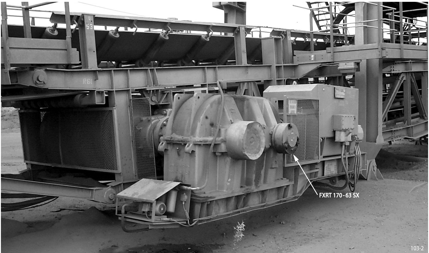
Iron ore conveyor plant in South Africa driven by three gear reducers with RINGSPANN backstops FXRT 170 SX.
